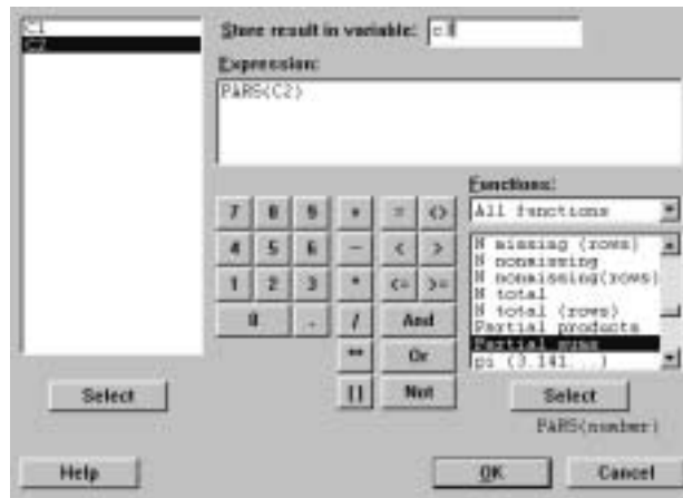
Display 4.1: Dialog box for computing partial sums of entries in C2 and placing these sums in C3.
